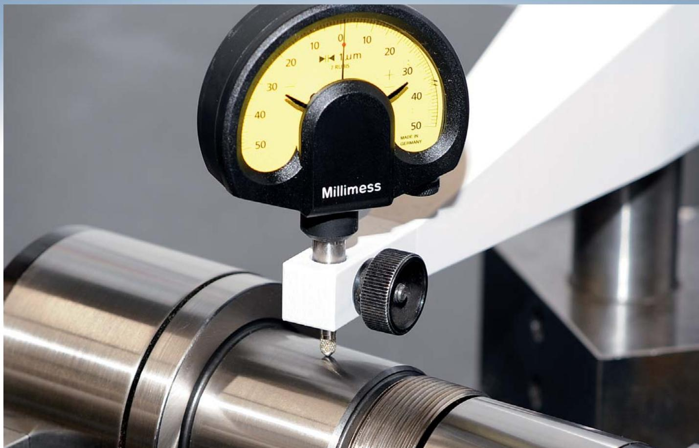
A spindle unit is subject to extremely high loads and requires optimized service in the event of a repair. Each spindle is carefully removed to localize the cause of the failure.
