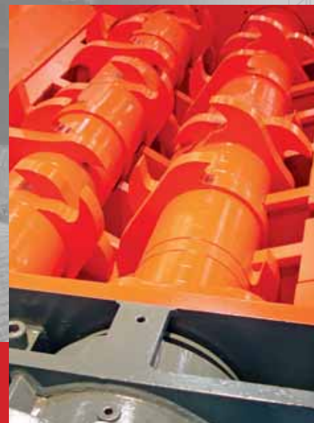
Shaft bearings located outside
