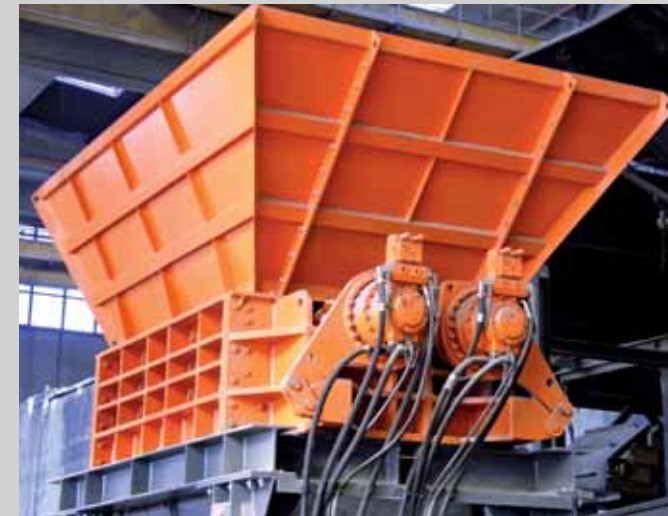
Shredding system for bulk waste
