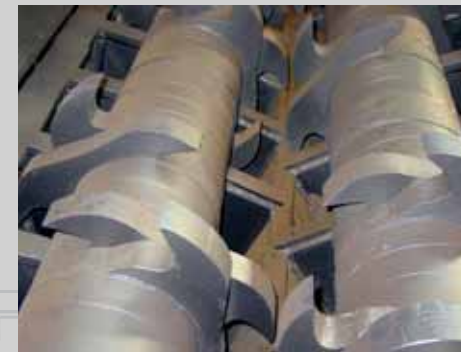
Cutting procedure running forward as well as reverse
