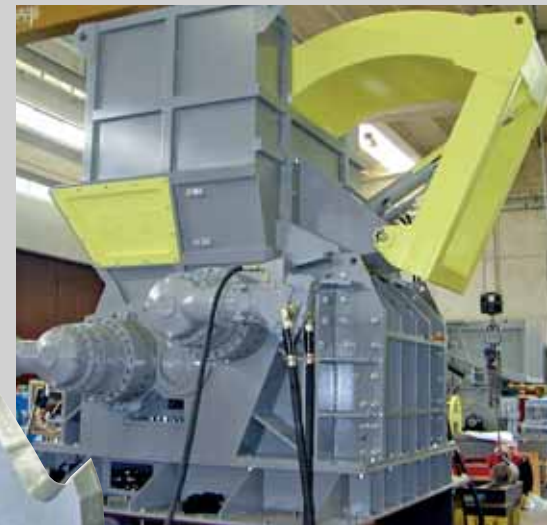
Shredding system for substitute fuels
