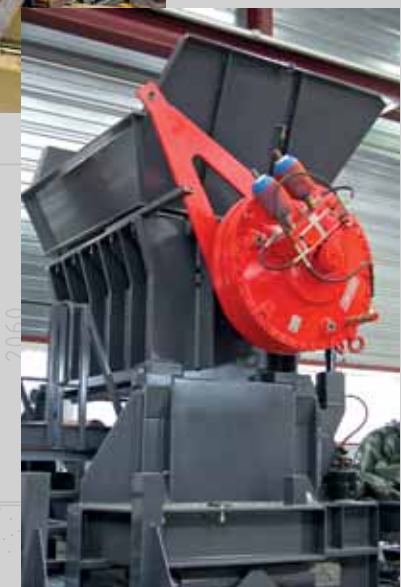
Granulator with hydraulic drive
