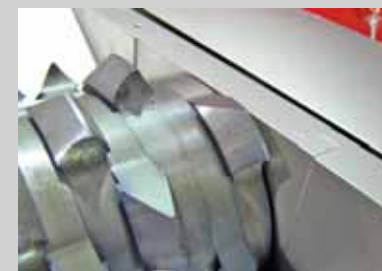
Quickly replaceable cutting rotor
