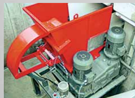
Centralized swarf shredding plant
