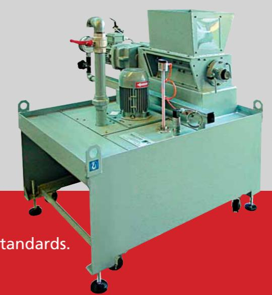
Single-shaft swarf shredder mounted on a small pump container.
