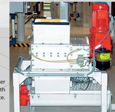
2-shaft swarf shredder as single machine with screw extraction gate.
