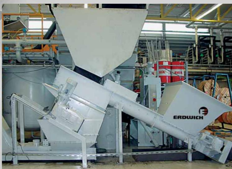
Central swarf reprocessing with swarf container feeder – double screw conveyor with bar sieve for discharge of foreign substances, 2-shaft swarf shredder and conveying system.
