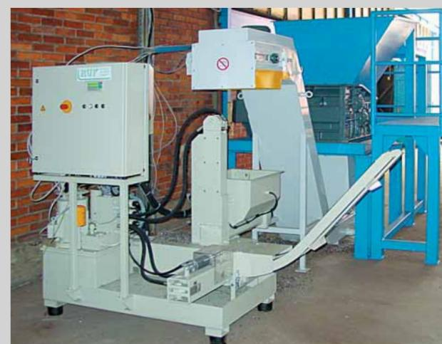
Central swarf reprocessing with swarf container feeder – 2-shaft swarf shredder with conveying system and briquetting press.
