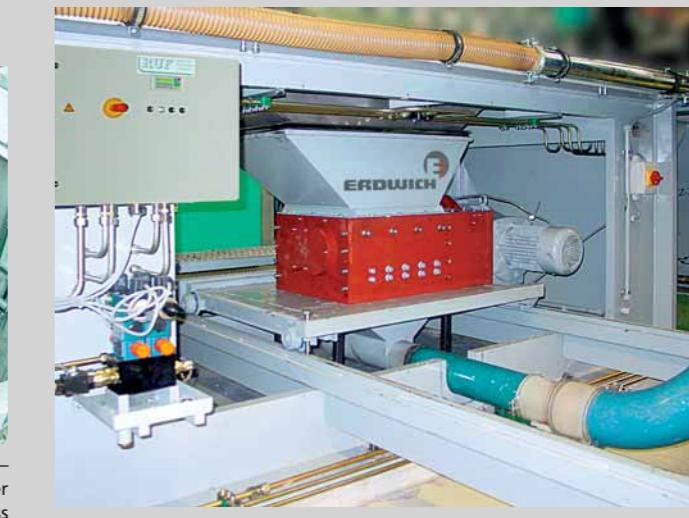
Decentralised swarf reprocessing – 2-shaft swarf shredder with extraction funnel placed directly under the machining centre. Can be drawn out on roller rack for revision purposes.
