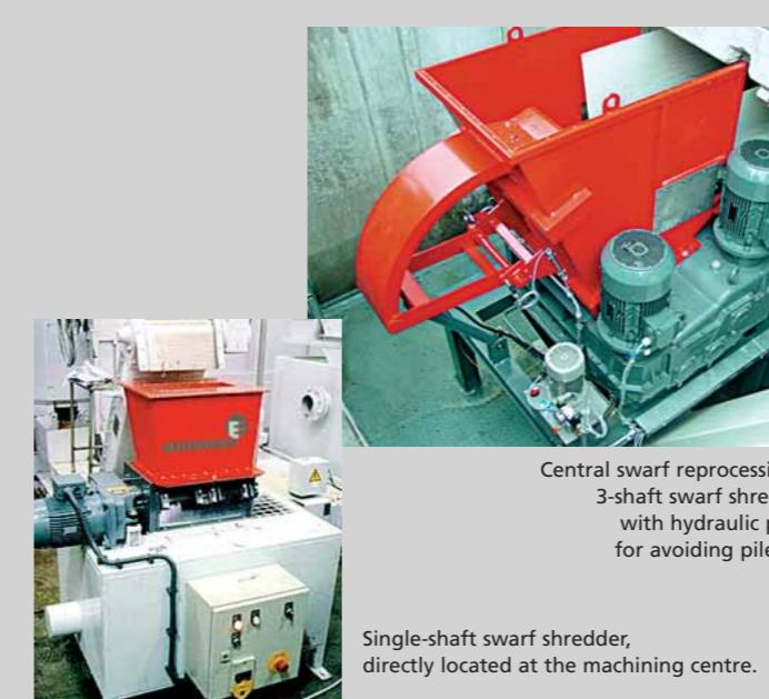
Central swarf reprocessing – 3-shaft swarf shredder with hydraulic press for avoiding pile-up.
